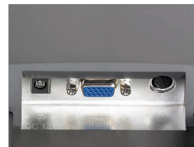
TS-15S provides dual serial touch interface for RS-232 and USB
