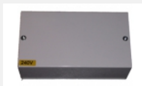
SNCA-PS24-4E An external power supply with one 4 Amp 24V AC fused output. Polycarbonate IP66 rated enclosure suitable for outdoor use.
