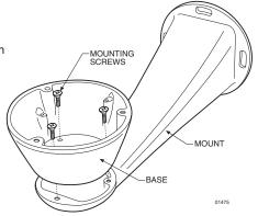
Route the wires and cables through the center of the Esprit mount. Reinstall the transformer module into the base. The transformer module can be positioned in the mount base in only one orientation.
