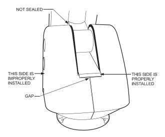
To reinstall the pan and tilt cover, do the following:
