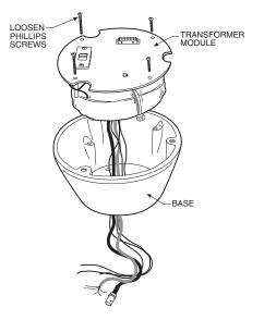
Attach the base of the system to an Esprit mount (EWM or EPP) with the three flathead 10-32 x 1/2-inch screws and washers (supplied).
