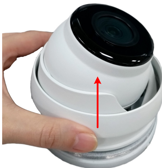
Remove the Outer Housing
