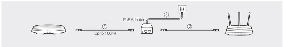
1. Connect the Ethernet cable from the Ethernet port (ETH1) of the EAP device to the provided PoE adapter's PoE port.
