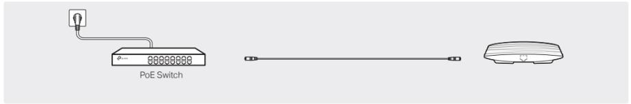
Connect an Ethernet cable from the PoE switch to the Ethernet port (ETH1).
