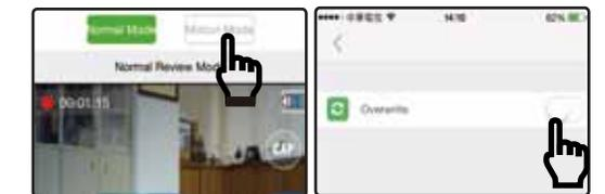
To overwrite recording, tap on "SETUP", which is at the top right corner of the live view screen, to enable or disable Overwrite recording.
