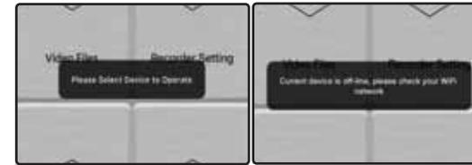
1. The Wi-Fi function on the device isn't turned on. To solve this please make sure the Wi-Fi function of the device is turned on.
