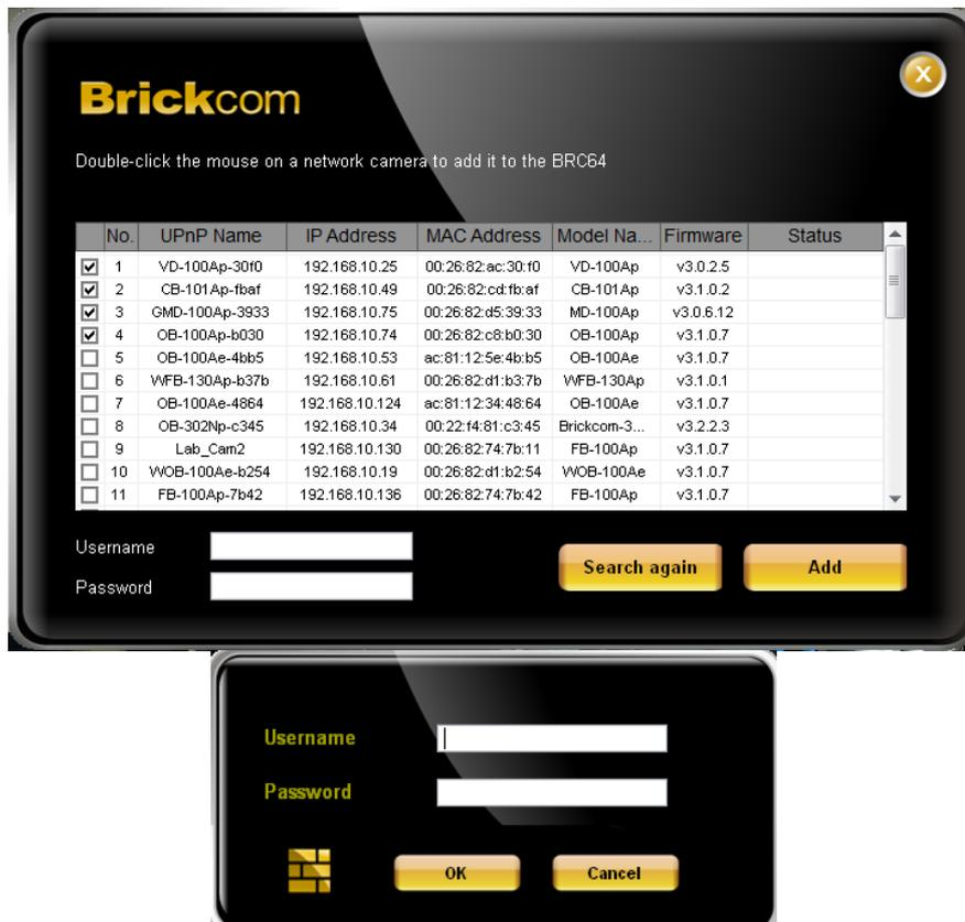
Click and select the Network Camera from the survey list. Enter the user name, password and select the stream type from the drop-down menu. For first time use of an IP camera, the user name and password are 'admin/admin'.
