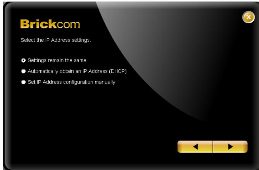
5. For configuring the IP address settings, select either <Settings remain the same>, <Automatically obtain an IP Address (DHCP)> or <Set IP Address configuration manually>. The DHCP setting is recommended.
