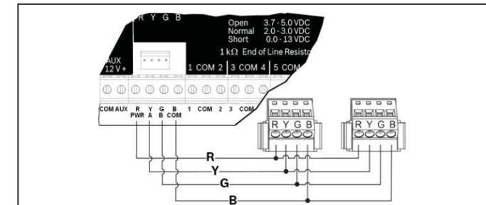
Figure 3.2: Installing multiple keypads using the SDI2 terminals
