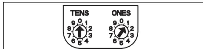
Figure 2.4: Address switches
