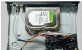
3. Place the HDD onto the bottom of the machine.
