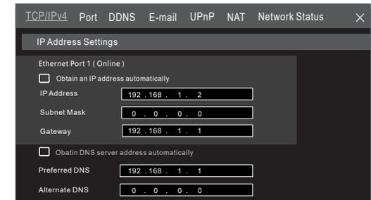
4. Go to Start → Settings → Camera → Add Camera. The DVR will automatically refresh the cameras searched. The IPC which supports the Onvif protocol may be added manually. If the IPC searched is not in the same local network as the DVR, you should select the device and click to modify the IP address.
