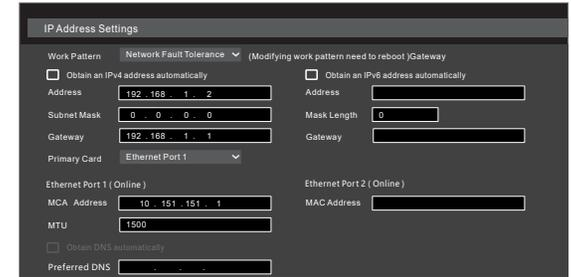
4. Go to Start → Settings → Camera → Add Camera. The NVR will automatically refresh the cameras searched. The IPC which supports the Onvif protocol may be added manually. If the IPC searched is not in the same local network as the NVR, you should select the device and click [ ] to modify the IP address.
