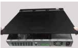
6. Install the cover back and fix it.
