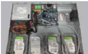
4. Install the other three HDDs according to above-mentioned method.
