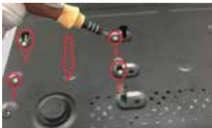
3. Turn over the machine and place the HDD with two screws onto the bottom of the case. Then lock the screws according to the order of the marks.
