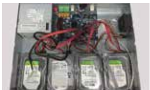
5. Connect the power and data cables.
