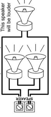
**Two 8 Ohm Speakers in Series (16 ohm load)**
