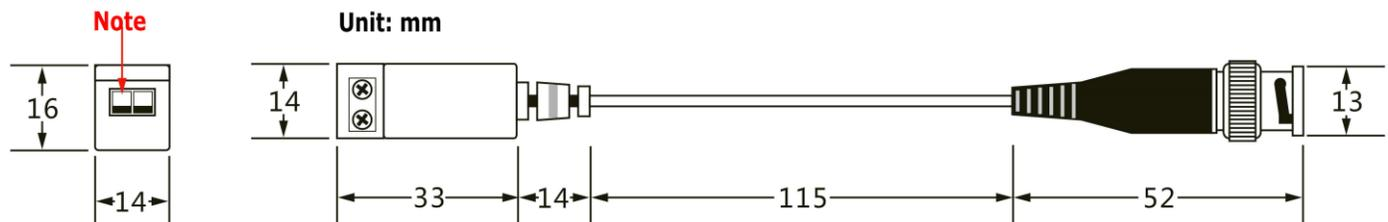
**Note:** This connection is with screw terminals. Recommend the cable  $>0.18\text{mm}^2$  ( $<1\text{mm}^2$ ).
