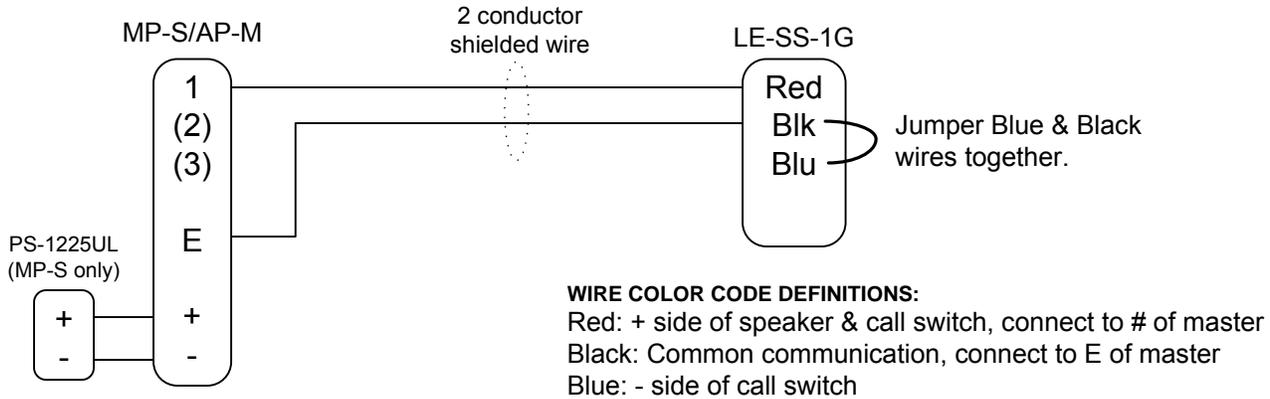
Intercom wiring must be run at least 20" away from any AC wiring, fluorescent lighting, dimmer switches, or any other electronic device that may cause interference.
