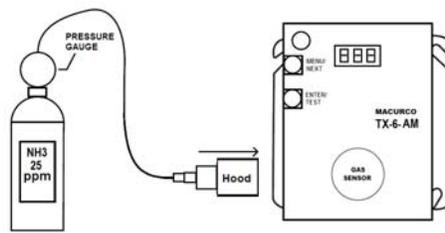
5. Turn on the regulator to start the gas flow and wait with the gas applied continuously.
